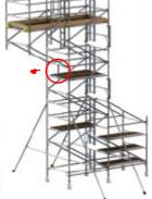
Fit the trapdoor deck and fixed deck on the fourth rungs of the tower, ensuring the decks are positioned each side of the 0.5m vertical brace as shown. The trapdoor deck must be oriented such that the trapdoor opens towards the outside of the structure. Ensure the deck wind-locks are engaged.
