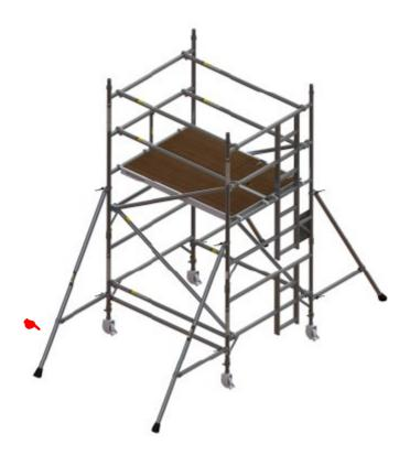
Fit two castors with adjustable legs to the 4 rung span frame and link to the main frame using 1.8m horizontal and 2.1m diagonal braces. Fit fixed decks as shown to support ballast, refer to table below. Level the whole assembly and ensure castors are locked. Ensure all wind-locks are engaged.
