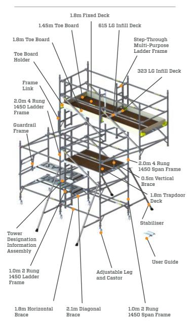
BoSS extended end 1.8m cantilever tower scaffold -1.8m long main tower with 1.8m long cantilever
