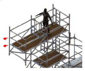
Fit the 0.3m and 0.6m infill decks. Fit toe board holders and toe boards around edges of top decks, as shown. Temporary guardrails to be stored in positions shown.
