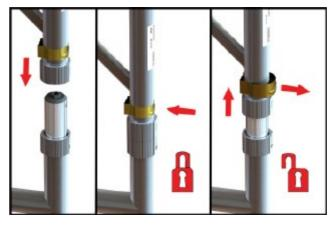
Ensure interlock clips on frame members are in the 'locked' position.
