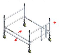
Fit the 4 rung ladder frame and the rung span frame to the structure base. Fit the 0.5m vertical brace into the span frame between its second and third crossbars at mid span as shown. Fit four diagonal braces in positions shown.
