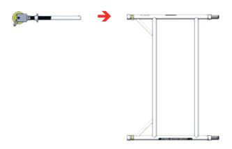
2 Fit one horizontal brace (red catch) onto the vertical of the 2 rung span frame, just below the bottom rung with the open section of the claw facing outwards.
