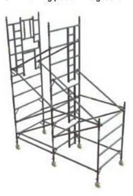
Build pattern - type 2 Tower working platform heights: 3.7m, 5.7m
