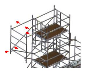
From the protected position within the main tower, fit two fixed decks. Fit two horizontal braces in positions shown. Ensure all wind-locks are engaged.
